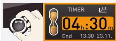
2. Turn the turn control until the desired duration is displayed.
