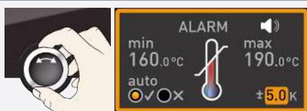
8. With the turn control, select the required tolerance band.
