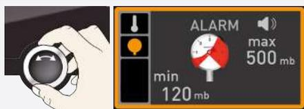
2. Turn the turn control until the pressure setting ● is highlighted.
