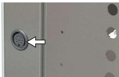
The 8-pin switching output on the rear right post is used to control the vacuum pump of the optional pump module (PM) via the vacuum oven (VO). The switching output is downward-compatible with the 3-pole contact of older pump modules. For this purpose, plug the 3-pole cable into the 8-pole contact.
