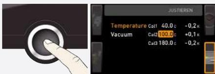
2. Press the confirmation key repeatedly, until the calibration temperature Cal2 is highlighted.
