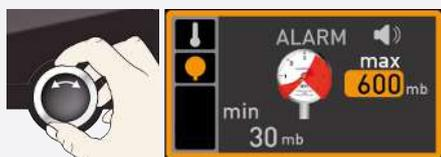
6. By turning the turn control, set the required upper alarm limit, 600 mbar in the example on the right.
