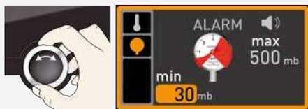
4. By turning the turn control, set the required lower alarm limit, 30 mbar in the example on the left.
