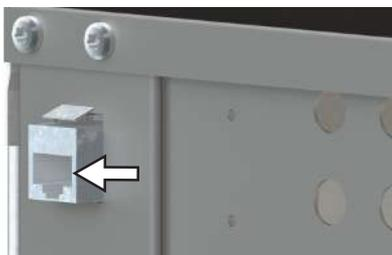
The unit can be connected to a network via the Ethernet interface, so that you can transfer programmes created with the AtmoCONTROL software to the unit and export logs.
