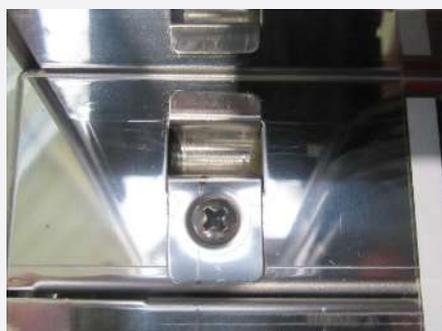
1. Loosen the Phillips screw of the locking bolt holder on the lower cross frame with a screwdriver.
