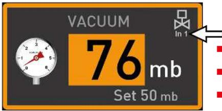
The display In1/In2 top right (arrowed, only for Premium VO49 and 101) indicates which gas connection is currently active:
