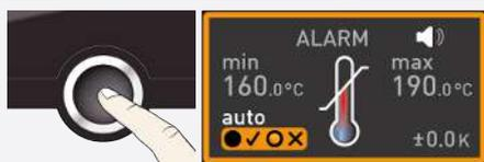
5. Press the confirmation key to apply the setting for the upper alarm limit.
