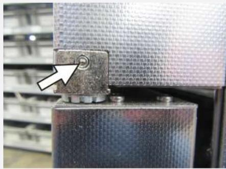
1. Open set screw on the front of the door hinge with an Allen key (size 2).
