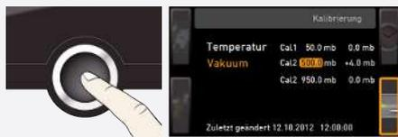
4. Press the confirmation key repeatedly, until the calibration point **Cal2** is highlighted.
