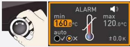
2. By turning the turn control, adjust the desired lower alarm limit.
