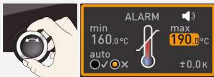
4. By turning the turn control, adjust the desired upper alarm limit.
