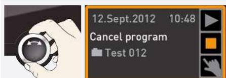
2. Turn the turn control until the stop symbol ■ is highlighted.
