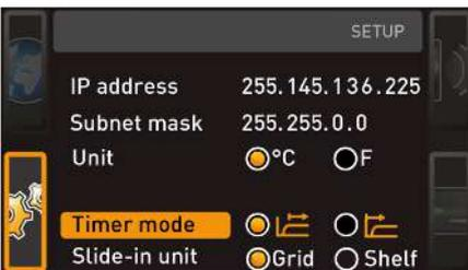
Here, you can choose whether the digital backwards counter with target time setting (see ▶6.5.2 Digital Backwards Counter) should be setpoint-dependent or not – in other words, whether the timer should not start until a tolerance band around the setpoint temperature is reached ⊕ or if it should start right after activation ⊙.
