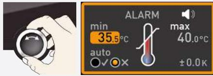
3. By turning the turn control, adjust the desired lower alarm limit.
