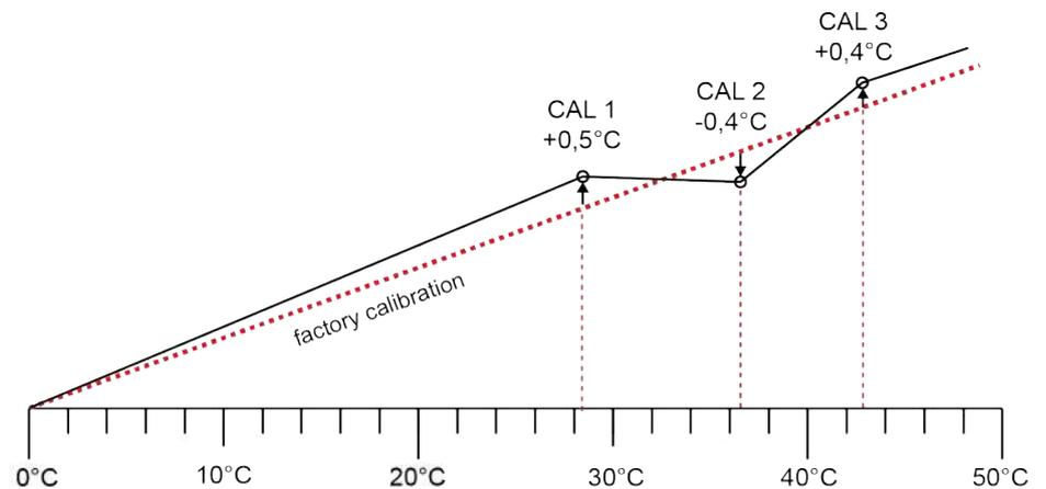
Example: Temperature deviation should be corrected
