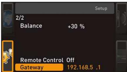
The Gateway setup entry is used to connect two networks with different protocols. The gateway is set the same way as the IP address (see ▶8.3.2 IP Address and Subnet Mask).
