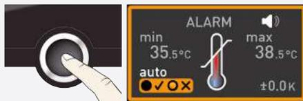
6. Press the confirmation key to apply the setting for the upper alarm limit.
