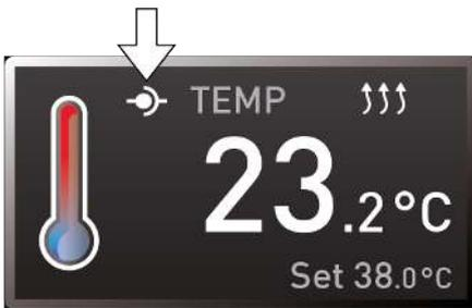
When the appliance is in remote control mode, the
