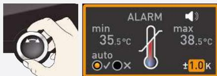
9. With the turn control, select the required tolerance band.
