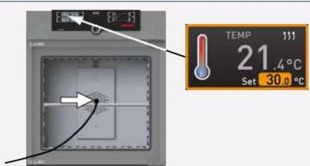
7. Position the sensor of a calibrated reference instrument centrally in the working chamber of the appliance.
