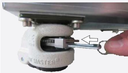
4. In the end position, push the ratchet lever in again to fix the foot.
