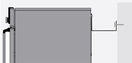
2. Bend the anti-tilt bracket up by 90° to achieve the required clearance from the wall (observe the minimum clearance).
