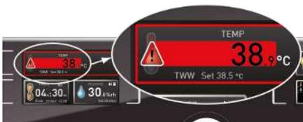
If temperature monitoring has been triggered, this is indicated by the temperature display: the actual temperature is highlighted in red and a warning symbol is shown. The type of temperature monitoring that has been triggered is shown beneath the temperature (see ▶ 7 Malfunctions, Warning and Error Messages).
