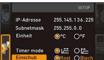
Here, you have to set the type of shelf (grid or metal panel) used. The selection **Metal panel** enables you to adjust the closed-loop control function to the different air flow characteristics in the chamber when using optional shelves instead of the grids provided as standard.
