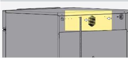
1. Screw the anti-tilt bracket to the back of the appliance as illustrated.
