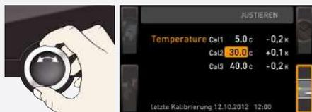
3. With the turn control, set the calibration temperature Cal2 to the specified temperature.
