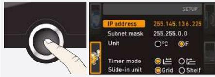
5. After setting the last three digits, confirm the new IP address by pressing the confirmation key.
