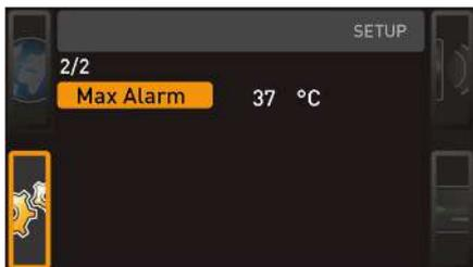
Here, you can set the trigger temperature of the automatic temperature monitoring system.
