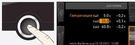
2. Press the confirmation key repeatedly, until the calibration temperature Cal2 is highlighted.
