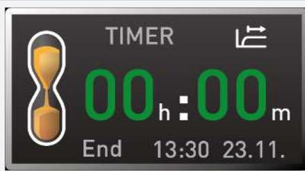
Once the timer has elapsed, the display shows 00h:00m.
