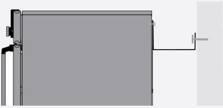
2. Bend the anti-tilt bracket up by 90° to achieve the required clearance from the wall (observe the minimum clearance).
