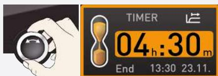
2. Turn the turn control until the desired duration is displayed.
