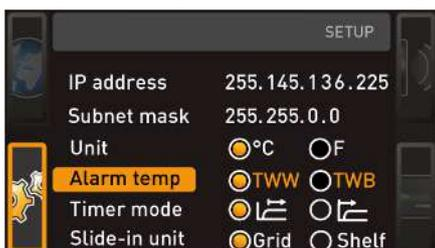
Here, you can choose which temperature protection class in accordance with DIN 12 880:2007-5 should be used (TWW or TWB, description from ▶6.6 Monitoring Function).
