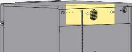
1. Screw the anti-tilt bracket to the back of the appliance as illustrated.
