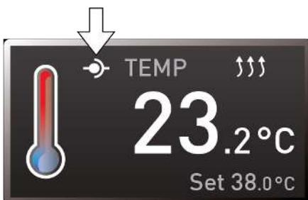
When the appliance is in remote control mode, the symbol appears in the temperature display.
