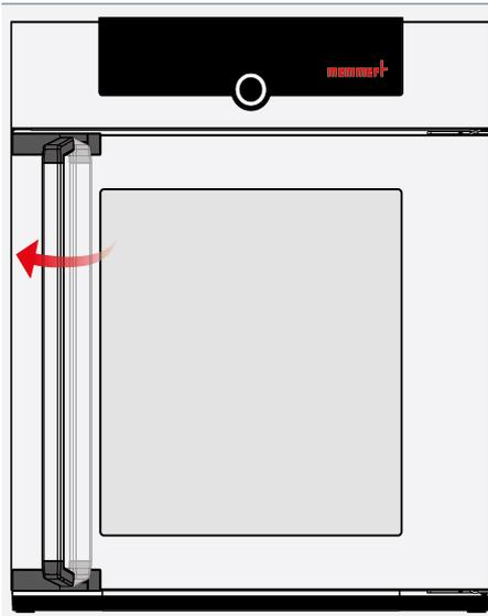
2. To close the door, push the door closed and push the door handle to the side.
