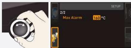
8. With the turn control, select the desired new trigger temperature.
