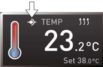
When the appliance is in remote control mode, the
