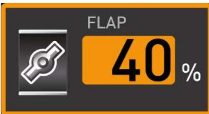
Setting range: 0% (closed, recirculating operation) up to 100% (fully open, fresh air operation) in 10% increments.
