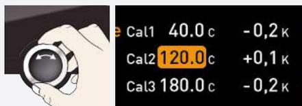
3. With the turn control, set the calibration temperature Cal2 to the specified temperature.
