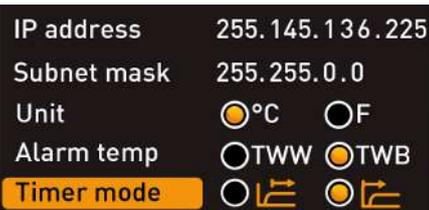
Here, you can choose whether the digital backwards counter with target time setting (see ▶6.5.2 Digital Backwards Counter) should be setpoint-dependent or not – in other words, whether the timer should not start until a tolerance band around the setpoint temperature is reached ⊕ or if it should start right after activation ⊙.
