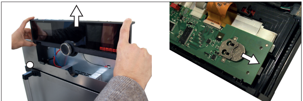
Fig. 22 Removing the lithium battery
