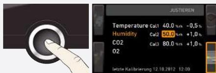
3. Press the confirmation key repeatedly, until the calibration point Cal2 is highlighted.
