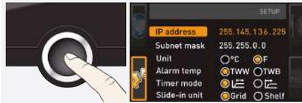
5. After setting the last three digits, confirm the new IP address by pressing the confirmation key.
