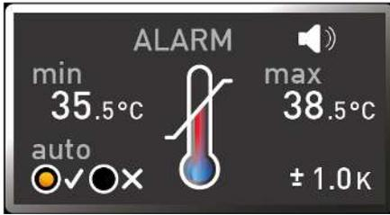
The electronic temperature monitoring measures the monitoring temperature via a separate Pt100 temperature sensor in the chamber. Temperature monitoring settings are made via the **ALARM** display. The settings made apply to all operating modes.
