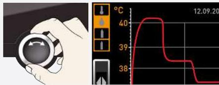
3. Select the humidity or a gas cylinder symbol with the turn control.
