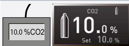
14. Compare the CO<sub>2</sub> value measured by the reference instrument with the CO<sub>2</sub> value displayed on the appliance.
