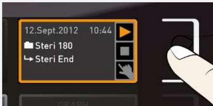
Once sterilisation is finished and the appliance has cooled down to 37 °C, end the sterilisation programme:
