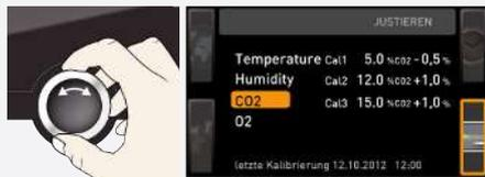
2. Turn the turn control until **CO<sub>2</sub>** or **O<sub>2</sub>** is highlighted.
