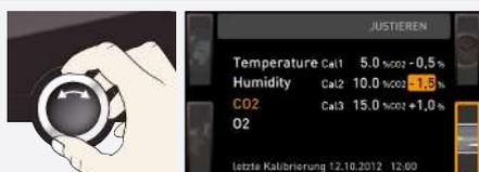
12. In the **SETUP**, adjust the calibration correction value **Cal2** to -1.5% (reference value measured minus value displayed).
