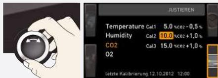
4. With the turn control, set the calibration point **Cal2** to 10%.
