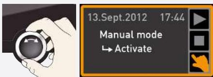
11. Turn the turn control until the hand symbol is highlighted.
