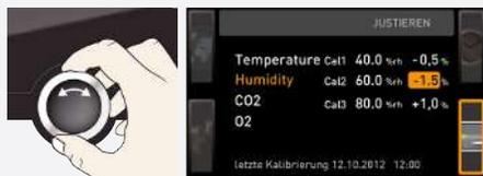
12. in the SETUP, adjust the calibration correction value Cal2 to -1.5% (actual value measured minus setpoint value).
