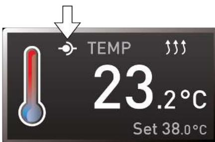
When the appliance is in remote control mode, the symbol appears in the temperature display.
