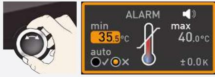
3. By turning the turn control, adjust the desired lower alarm limit.
