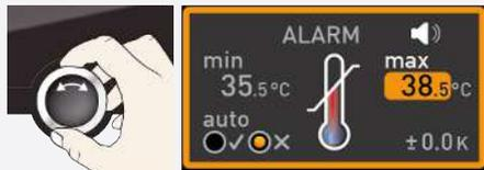
5. By turning the turn control, adjust the desired upper alarm limit.
