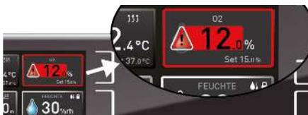
If O<sub>2</sub> monitoring has been triggered, this is indicated by the O<sub>2</sub> display: with the actual value on a red background accompanied by a warning symbol ▲.
