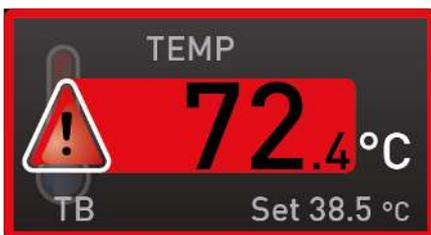
The appliance is equipped with a mechanical temperature limiter (TB) of protection class 1 in accordance with DIN 12880.
