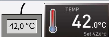
13. Compare the temperature measured by the reference measurement instrument with the temperature displayed on the appliance.
