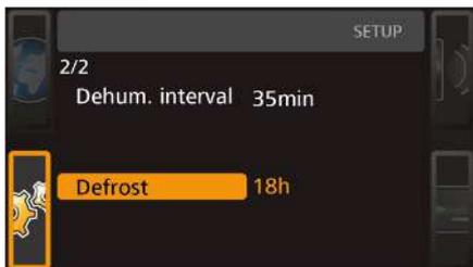
The integrated automatic defrosting system for the cooling unit ensures problem-free operation of the cooled incubator at low temperatures and in permanent operation. The defrosting interval can be set in 6-hour increments, between 6 and 48 hours. The **Off** setting deactivates automatic defrosting.
