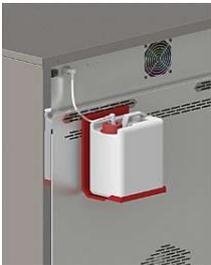
The water tank for size 750 appliances can be attached using the supplied mounting bracket. To do so, hook the tank mounting bracket into the slots on the rear of the appliance. For wall mounting, the tank mounting bracket also has two drill holes (fastening material not included).
