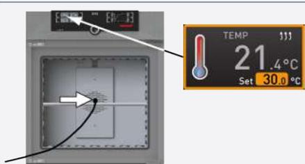
7. Position the sensor of a calibrated reference instrument centrally in the working chamber of the appliance.
