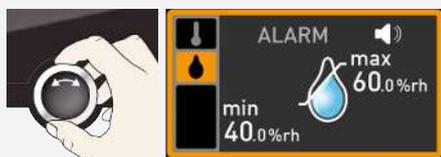
2. Turn the turn control until the humidity setting is highlighted.
