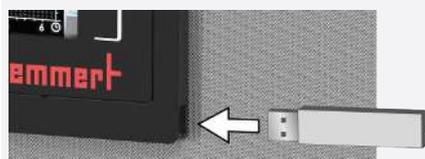
1. Connect the USB storage medium to the port on the right of the ControlCOCKPIT.
