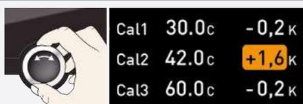
11. In the **SETUP**, adjust the calibration correction value Cal2 to the deviation temperature (actual value measured minus setpoint value).
