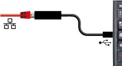
With an Ethernet to USB converter it is possible to connect the Ethernet connection of the appliance to the USB port of a computer/laptop.
