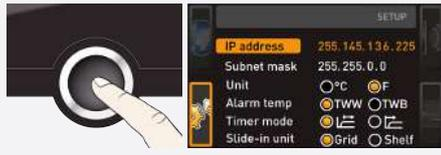
5. After setting the last three digits, confirm the new IP address by pressing the confirmation key.
