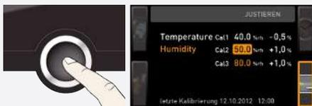
3. Press the confirmation key repeatedly, until the calibration point Cal2 is highlighted.
