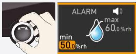
4. By turning the turn control, set the required lower alarm limit, 50% rh in the example on the left.
