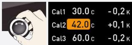
3. With the turn control, set the calibration temperature Cal2 to the specified temperature.
