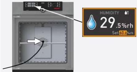
8. Position the sensor of the calibrated reference instrument centrally in the working chamber of the appliance.
