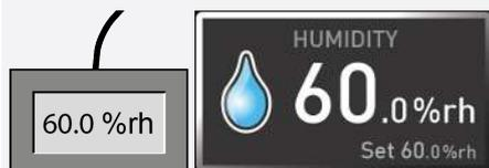
After the calibration procedure, the humidity measured by the reference instrument should now also be 60% rh.
