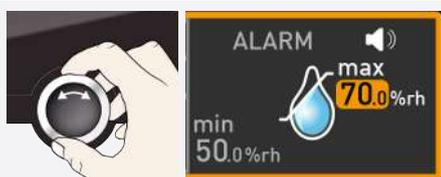
6. By turning the turn control, set the required upper alarm limit, 70 % rh in the example on the left.
