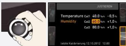
4. With the turn control, set the calibration point Cal2 to 60% rh.
