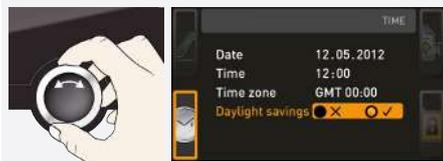
8. Set summertime to off (X) or on (✓) with the turn control – in this case on (✓).
