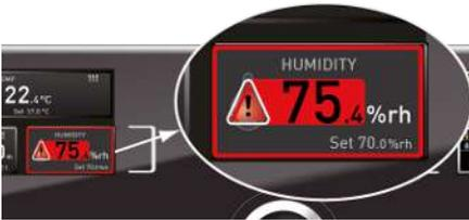
If humidity monitoring has been triggered, this is indicated by the humidity display: the actual humidity is highlighted in red and is accompanied by a warning symbol ▲.
