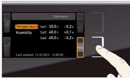
1. Press the activation key to the right of the **CALIB** display.
