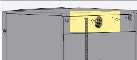
1. Screw the anti-tilt bracket to the back of the appliance as illustrated.
