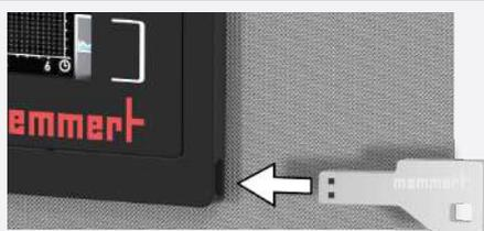
1. Insert the USB storage medium with the USER ID data into the USB port on the right of the ControlCOCKPIT.
