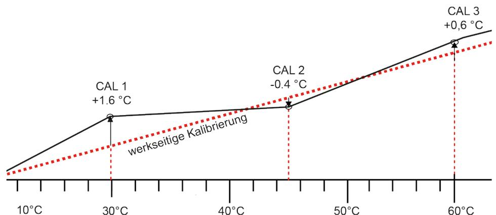
Example: Temperature deviation should be corrected
