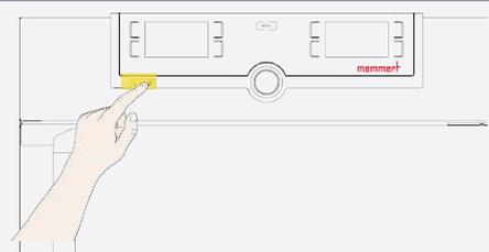
1. Switch off the active unit functions (reset setpoint values).
