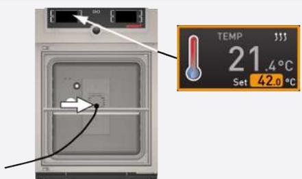
7. Position the sensor of a calibrated reference instrument centrally in the working chamber of the appliance.
