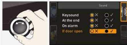
3. With the turn control, select the desired setting – in this example OFF (X).
