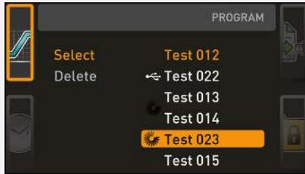
The name under which you save the program will be shown in the program selection view on the display of the appliance once it was transferred to the appliance (file name in the example to the right: `Test 023.atpro`).
