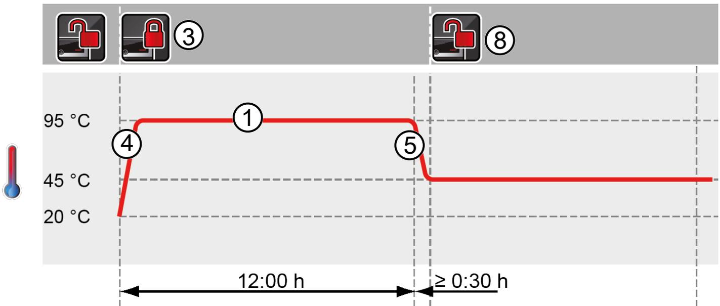
The door is locked at the beginning of the program ③. Then, the appliance heats up to 95.0 °C ④ and maintains this temperature for 12 hours ①. Subsequently, the temperature is lowered ⑤ for 30 minutes ② to 45.0 °C and then, the door is opened ⑧. The setting **SPWT on** ⑦ ensures that the door is opened only when the temperature really has dropped to 45.0 °C, even if this takes longer than 30 minutes. Below the temperature change is shown in K/min ⑥.
