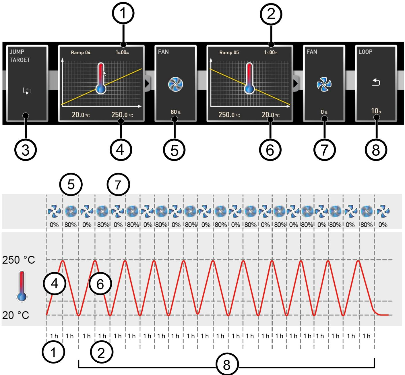
First, the appliance heats up to 250.0 °C ④ for one hour ①. Then, the fan begins to run at 80 % power ⑤ and the temperature is lowered for one hour ② to 20.0 °C ⑥. Subsequently, the fan is switched off ⑦. This sequence is repeated from the jump target ③ ten times ⑧.
