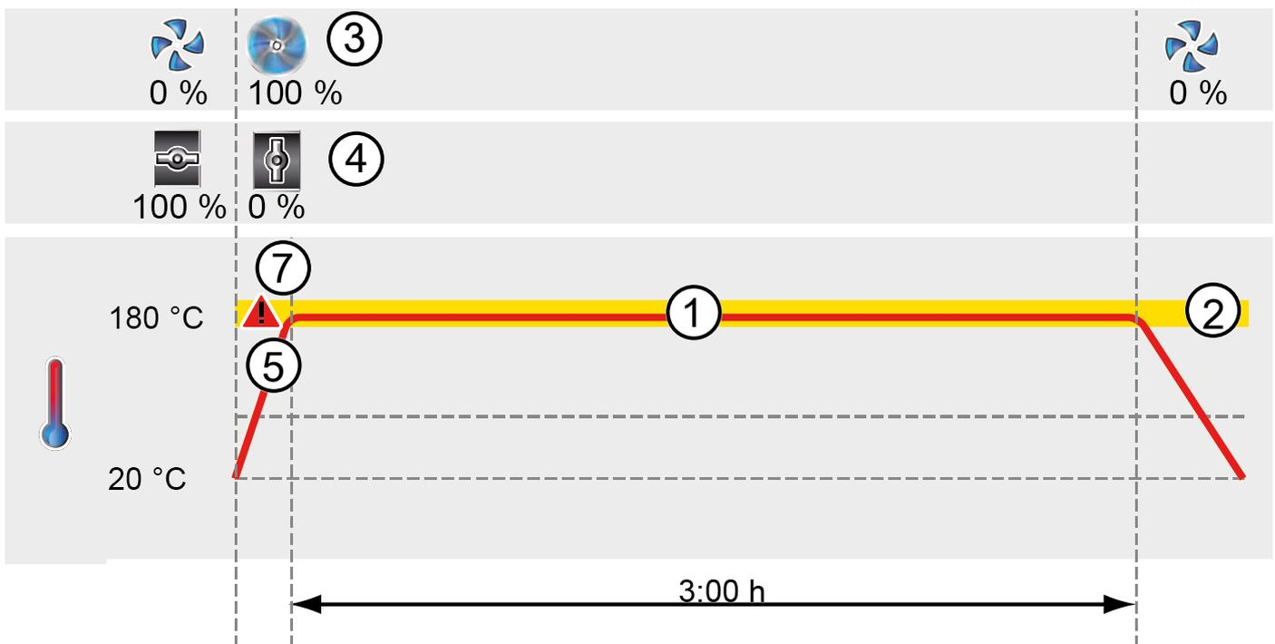
At the beginning, the fan is switched on to 100% ③ and the air flap is closed (0%) ④. Then, the appliance heats up to 180.0 °C ⑤ and maintains this temperature for 3 hours ①. The setting **Safe** ⑥ ensures that the sterilisation time does not start ⑦ before the set tolerance band ② is reached and is restarted if it is exceeded.
